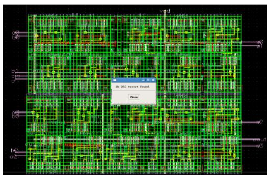
Fig.4.8. CSLA using CBL with DRC errors cleared.
