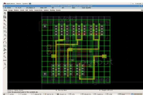
Fig.4.6. Layout of MUX.
